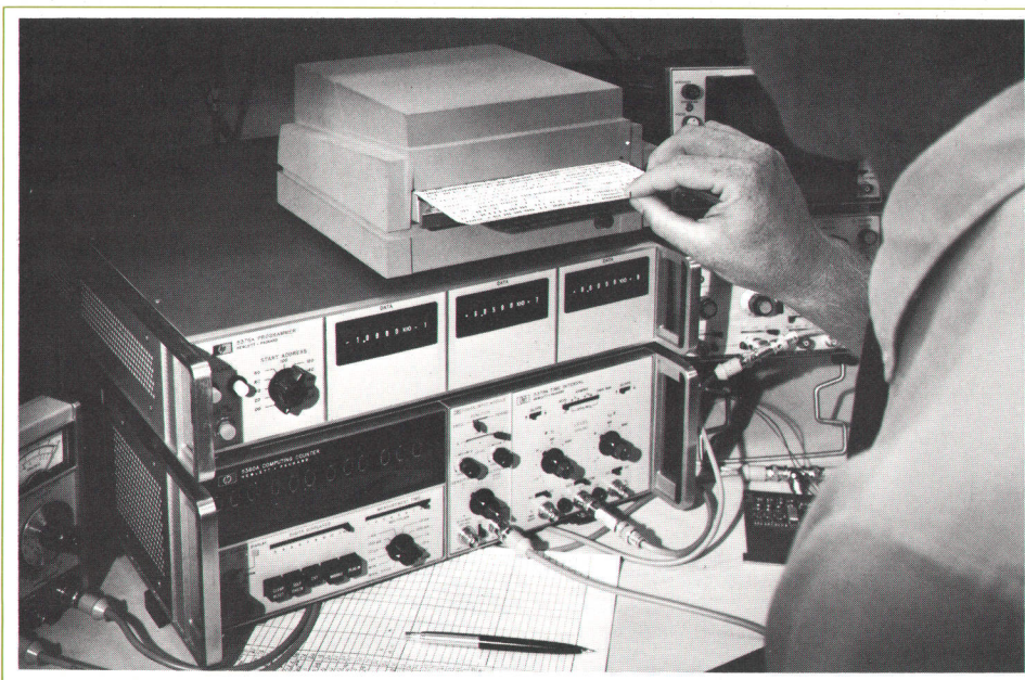
Fig. 2. A new modular systems programmer, Model 5376A, is the cornerstone of computing-counter systems. It is programmed by plug-in diodes or by punched card. Details are in the article on page 7.
